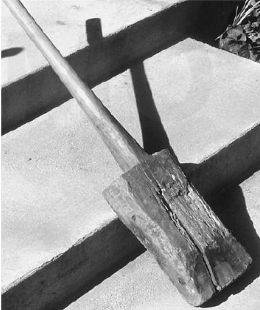
5-3. A wooden tamper used to compact mud in pisé construction in northern Peru (photo by the author, 1985).
